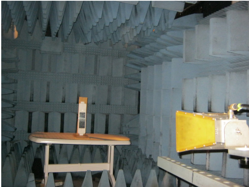
Figure 5. Radiated Emission Test Above 1 GHz
