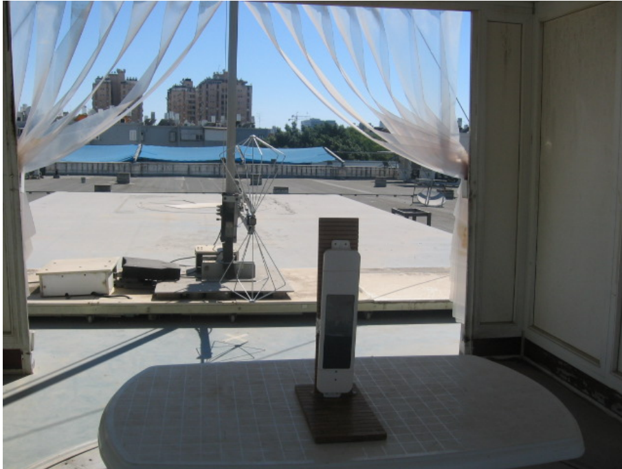
Figure 3. Radiated Emission Test 30-200 MHz
